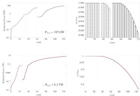
Figure 3: (top) Radiation power and RMS undulator parameter in start-to-end simulations of fresh bunch self-seeding at the LCLS and (bottom) for an optimized superconducting undulator design. The extraction efficiency is over 6 times the SASE saturation level in the LCLS case and in the superconducting undulator case reaches 12 %.
