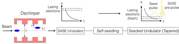
Figure 1: Schematic of the fresh bunch self-seeding experimental set-up with the geometry of the dechirper for the LCLS with a beam on and off axis. The experimental values for the gap and offset are:  $2a=4.5$  mm,  $y=1.7$  mm
