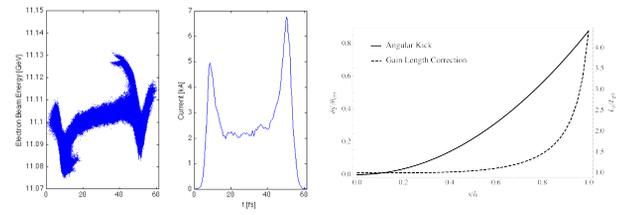
Figure 2: (left) Longitudinal phase space and current profile at the entrance of the undulator for the LCLS start-to-end beam from the particle tracking code ELEGANT. (right) Angular kick and gain length correction factor as a function of intra-bunch coordinate for the LCLS simulation case parameters (see Table 1). Note: head of the beam is at  $s = 0$ .
