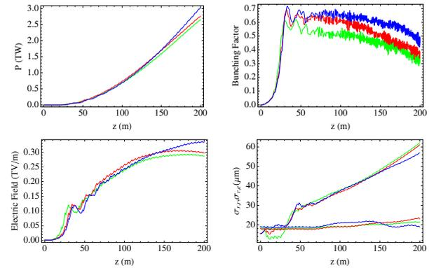
Figure 3: Comparison of time independent results for Gaussian (green), parabolic (red) and uniform (blue) transverse beam distributions at  $\lambda_r = 1.5 \text{ \AA}$ . X-ray pulse power, upper left and electric field, lower left, electron microbunching upper right, electron and radiation beam radii lower right.
