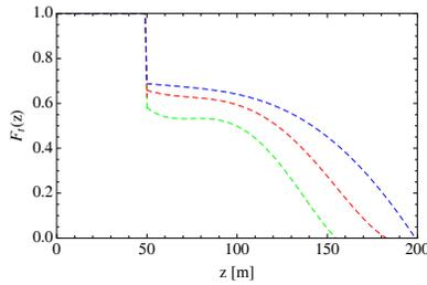
Figure 5: Evolution of the trapping function  $F_t(z)$  for the Gaussian (green), parabolic (red) and uniform (blue) transverse electron distributions obtained from GENESIS single frequency (solid) and time dependent (dashed) simulations.
