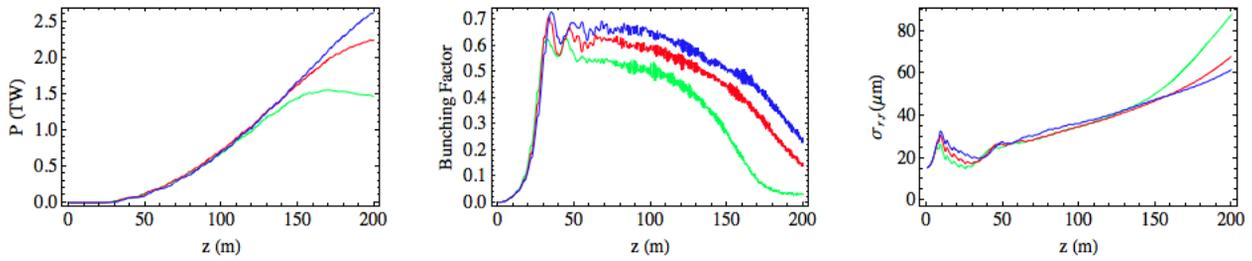
Figure 4: Power, bunching factor and radiation size as a function of longitudinal distance for transversely Gaussian (green), parabolic (red) and uniform (blue) beams. The results are shown for a wavelength  $\lambda_r = 1.5 \text{ \AA}$  and bunch length of 16 fs. The optimized taper profiles are found in time independent simulations.
